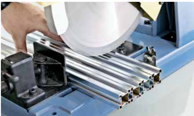
↑ Up to four Geberit GIS profiles can be cut to length at the same time with the chop saw.
